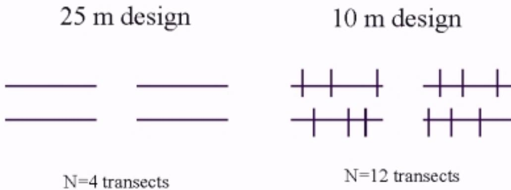
Figure 2. Design of permanent transects established at each site. **A.** H-shaped transect design created at each study site to conduct visual strip transects for fishes. Two 60 m transect tapes were positioned along six permanent stainless-steel eyebolts. Divers surveyed four 25 m transects separated by 10 m buffer areas between replicates. **B.** Alternate transects designs evaluated for benthic habitat sampling.
